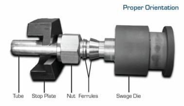
3. Insert tubing and swage die into Swaging head and pump to pressure for corresponding tube diameter:
