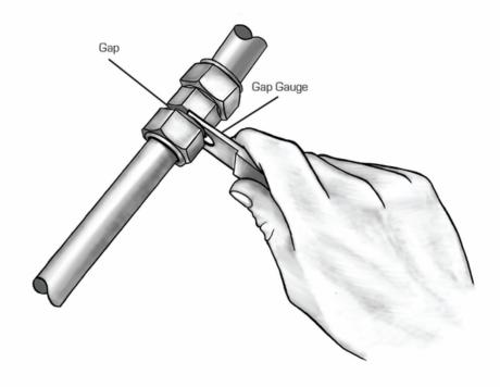
The gauge should NOT fit into the gap when tightened properly
